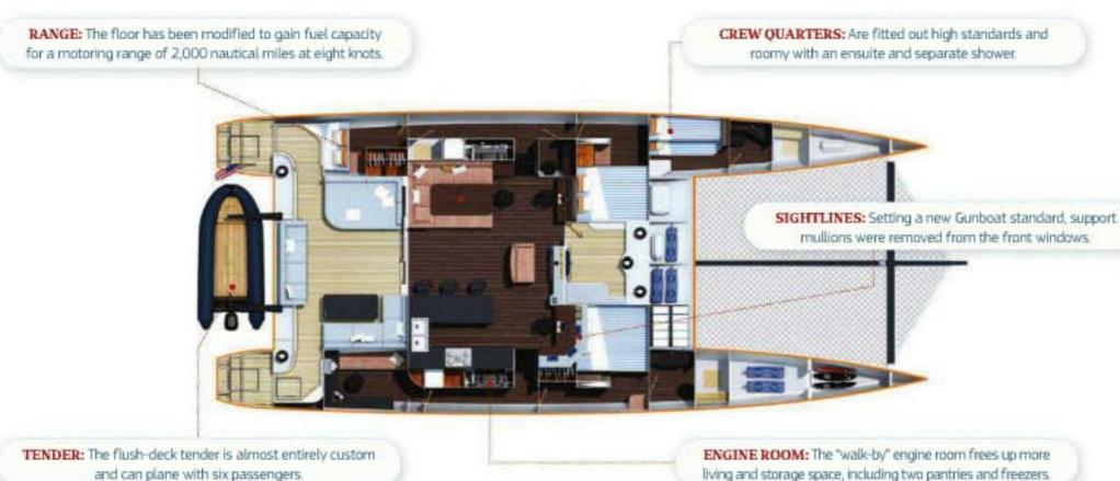
LOA: 65FT 11IN (201M) LWL: 62FT (18.9M) BOA: 28FT 3IN (8.6M) BEAM: 21FT 8IN (6.6M) DRAFT (BOARD DOWN/BOARD UP): 8FT 6IN (2.6M)/2FT 3IN (0.7M) DISPLACEMENT (LIGHT/MAX
